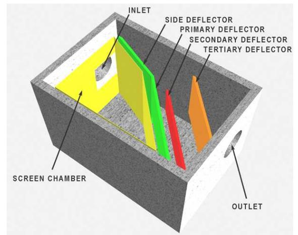
"NTVS, a unique trapping mechanism"
