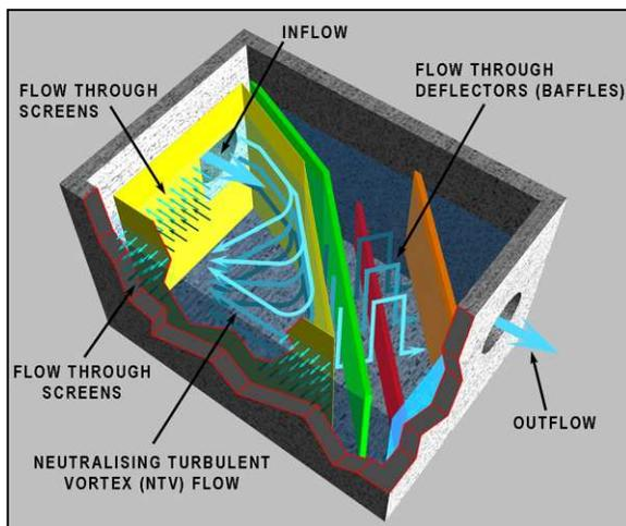
In the figure on the left, the water flow pattern is shown, demonstrating specifically the Neutralizing Turbulent Vortex (NTV) mechanism.
