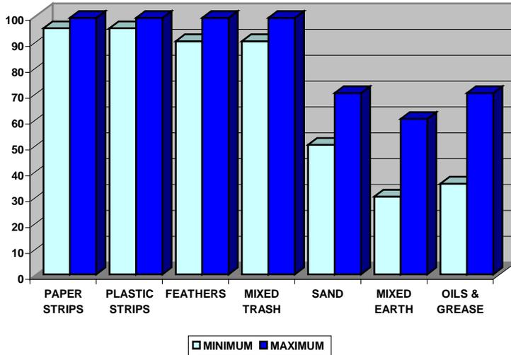
The adjoining figure shows the results from laboratory testing for a range of pollutant types and sizes. It shows that the NTVS achieves high capture efficiencies for a wide range of pollutants. However, it is important to note that factors, such as the range of flows monitored, the homogeneity of the pollutants, the quantity of previously captured material, and the accuracy in flow and material measurement, can present difficulties in accurately determining the capture efficiencies.
