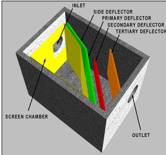
The figure on the left shows the general arrangement of the NTVS unit, consisting of an external shell, a screen chamber and four deflectors. Note that the unit is unsymmetrical, but the NTVS is equally applicable with its componential arrangement mirrored longitudinally.
