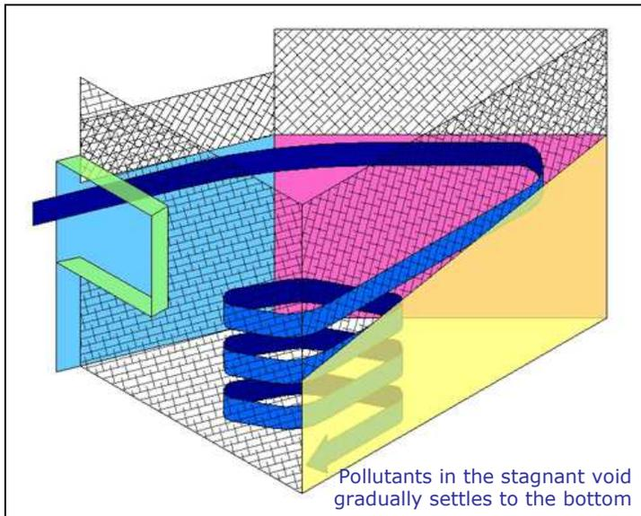
Due to the nature of the NTV flow, pollutants are pushed into the stagnant void created. Pollutants trapped in this area are virtually stationary and slowly settles towards the bottom of the NTVS unit.
